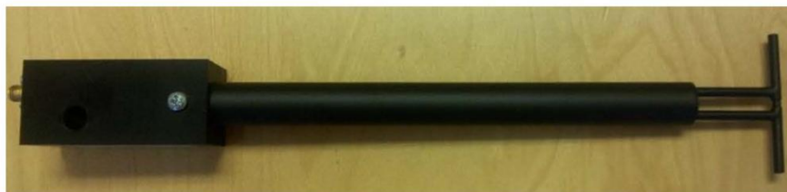
Figure 1 – MVG COMOSAR Validation Dipole
