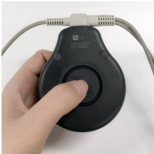
Figure 7-7 Testing a TOCO Transducer
