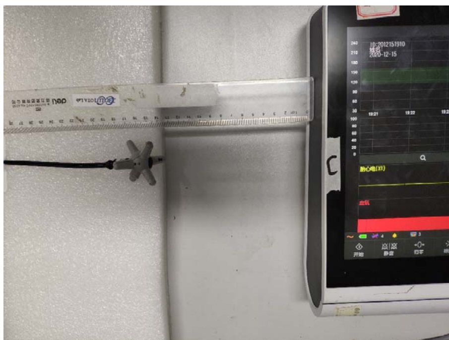
E-field Test Setup Photo of Position C(15cm)
