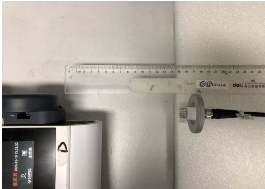
H-field Test Setup Photo of Position D(15cm)
