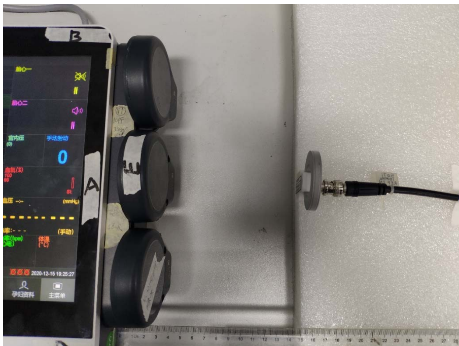
H-field Test Setup Photo of Position A(15cm)
