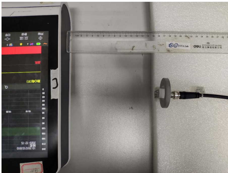
H-field Test Setup Photo of Position C(15cm)
