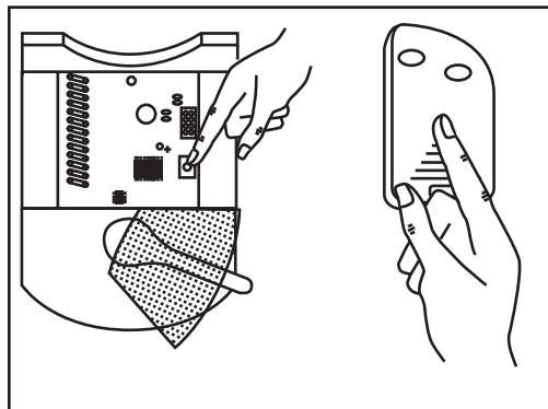
**THEN** Quickly press either button on remote. Hear 3 beeps.
