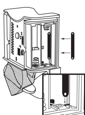
8. Then slide bars down through holes as far as possible, and install 4 AA batteries..
