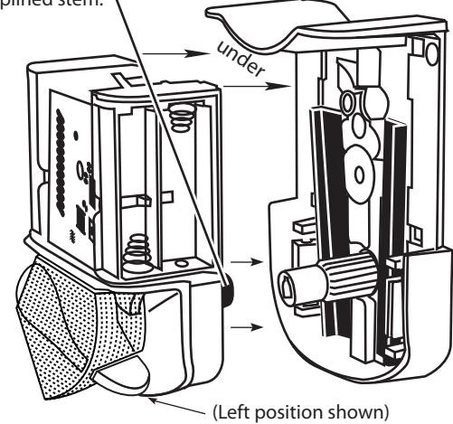
7. Insert black bars (in tiny grooves) in both left and right sides of gearbox.
