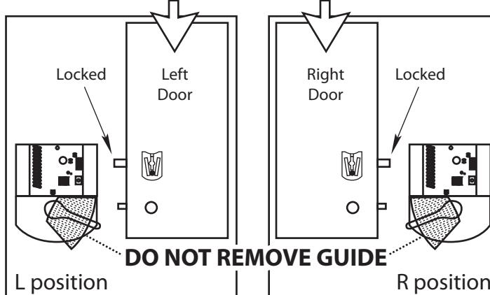
6. With door LOCKED, slide black tip on to splined stem **WHILE** guiding under top cap.
