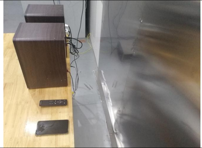
Conducted Emissions Test Setup Side View
