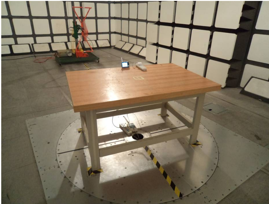
Radiated Emissions – Front View (30-1000 MHz)
