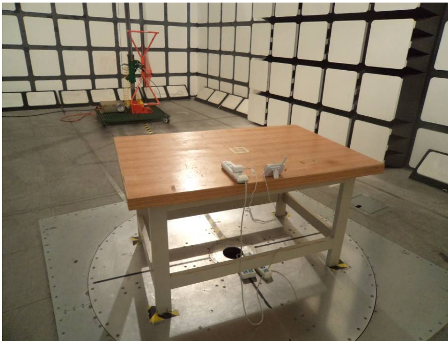
Radiated Emissions – Rear View (30-1000 MHz)
