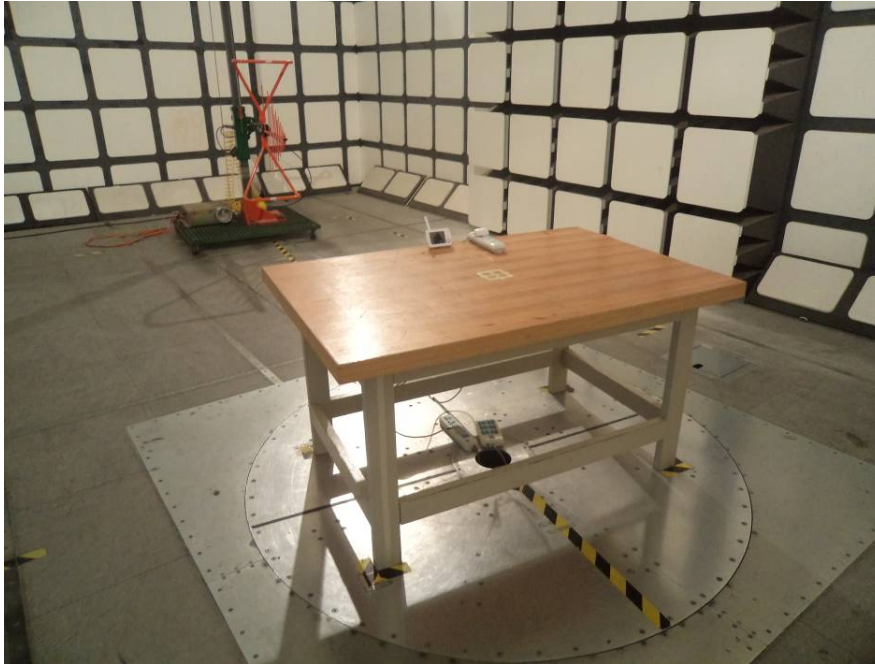
Radiated Emissions –Front View (Below 1 GHz)
