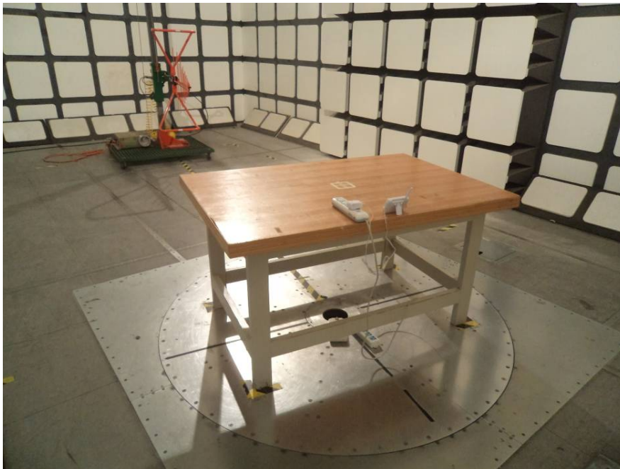
Radiated Emissions –Rear View (Below 1 GHz)
