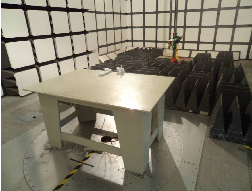
Radiated Emissions – Front View (Above 1 GHz)
