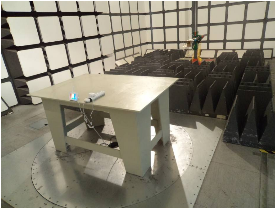
Radiated Emissions – Rear View (Above 1 GHz)
