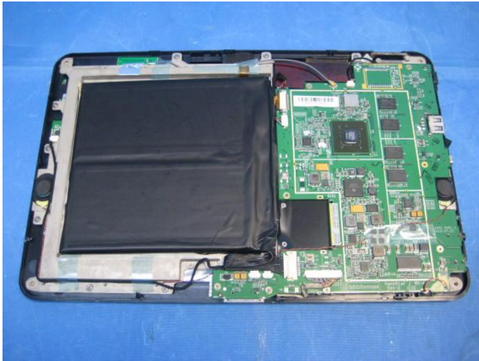
Structure 2: Without Shielded cover
