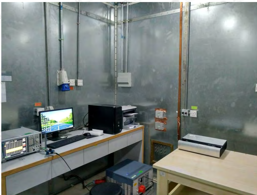
FCC RADIATED EMISSION TEST SETUP BELOW 1GHZ
