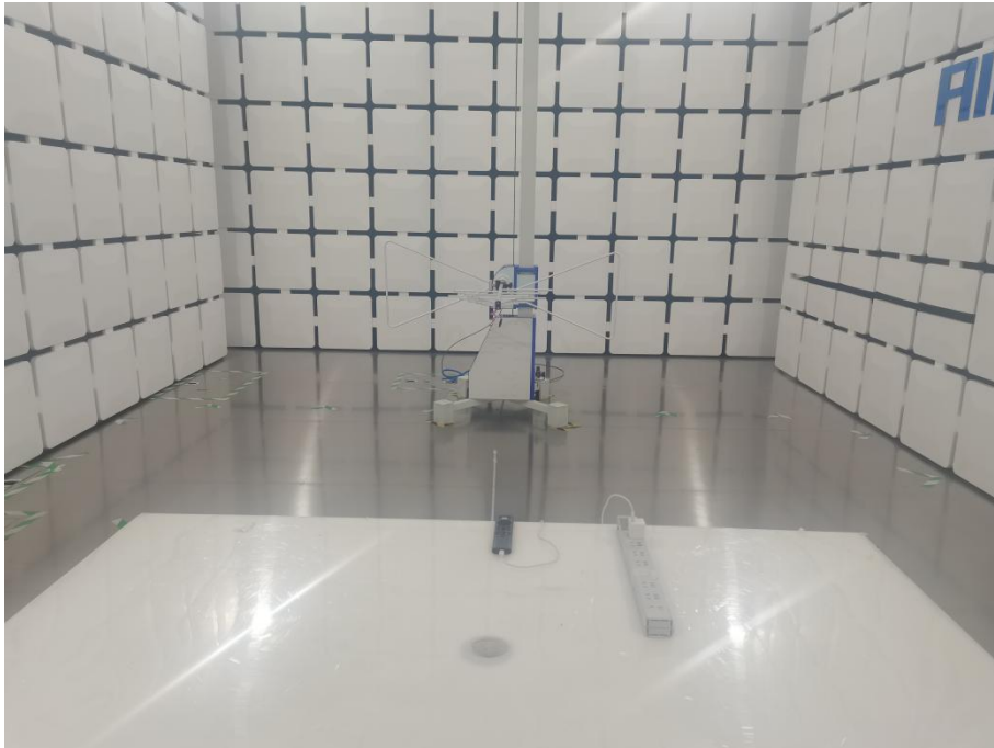
Radiated Measurement Photo (below 1 GHz)
