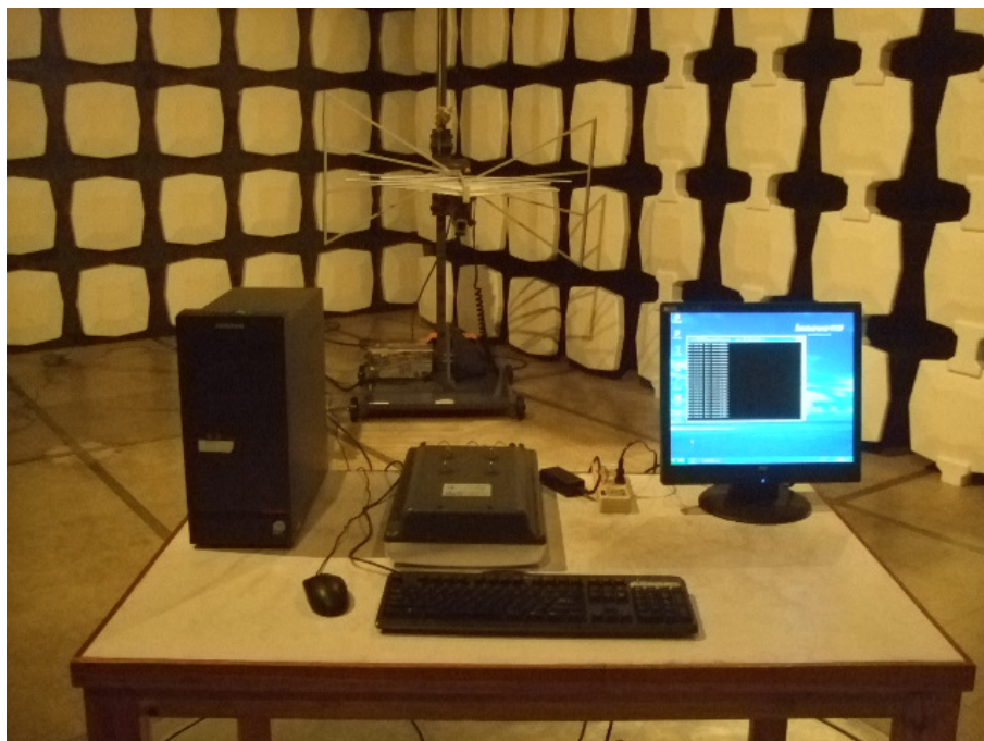
Radiated Emission Test Set-up -below 1GHz
