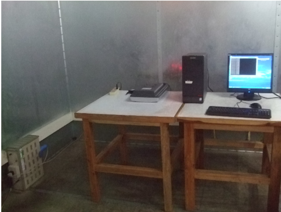
Conducted Emission Test Set-up-Front View
