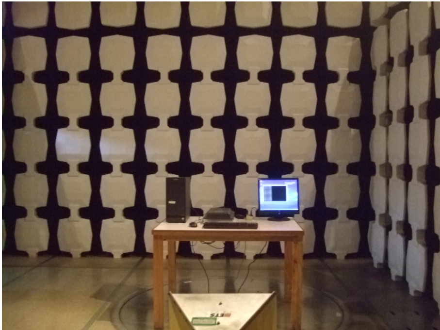
Radiated Emission Test Set-up - Above 1GHz
