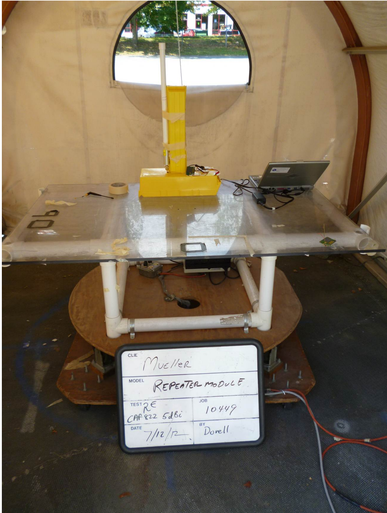
Figure 6- Set up for radiated emissions testing, front view
