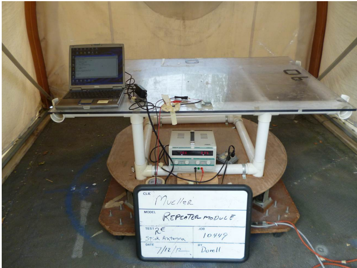
Figure 10- Set up for radiated emissions testing, front view
