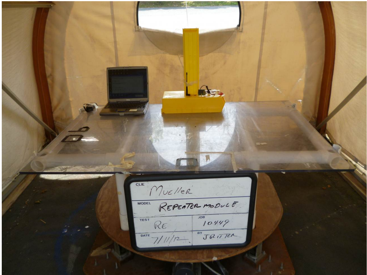
Figure 3 - Set up for radiated emissions testing, front view
