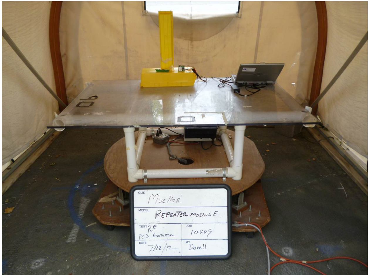
Figure 9- Set up for radiated emissions testing, front view
