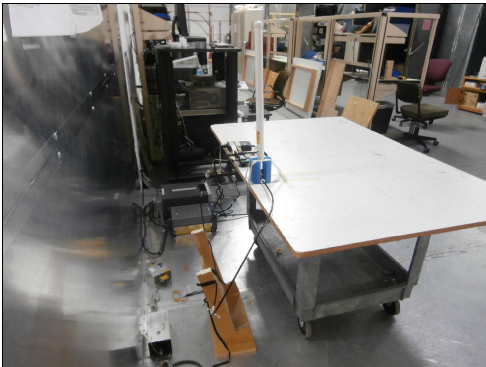
Figure 6: Conducted Emissions – Dipole Antenna
