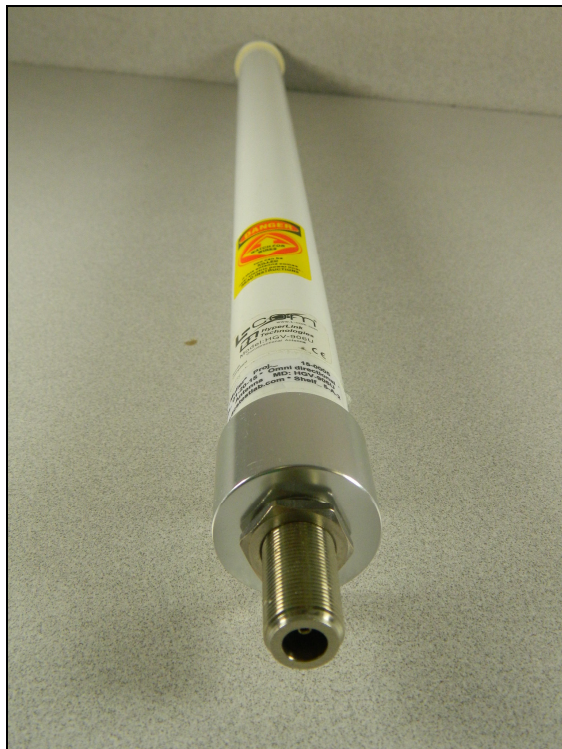
Figure 6: External Photo – Dipole Antenna
