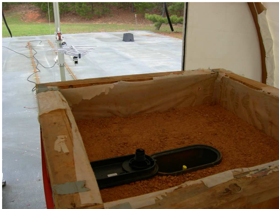
Figure 2: Radiated Emissions – Metal Pit with Composite Lid
