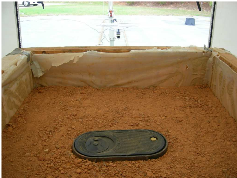
Figure 3: Radiated Emissions – Metal Pit with Composite Lid
