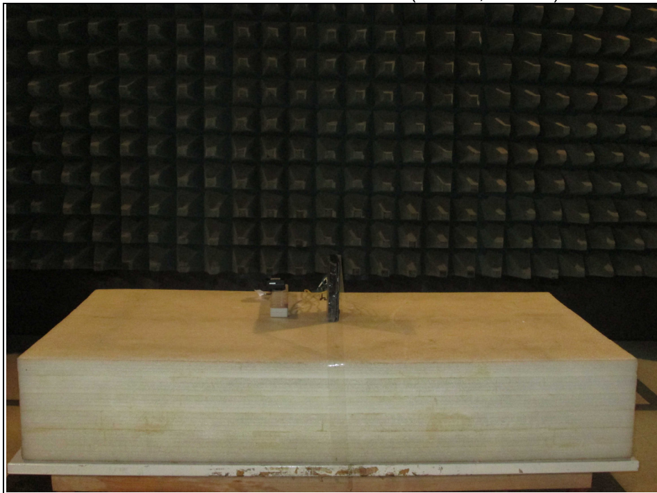
Radiated Emission Test below 1GHz (2.4GHz, Mode B)
