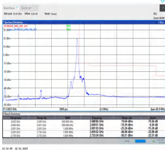
1-N41-PC3-30-40-H-5-CP-QPSK-Edge_1RB_Righ t-1@105-Ant1-1--PASS-see graph
