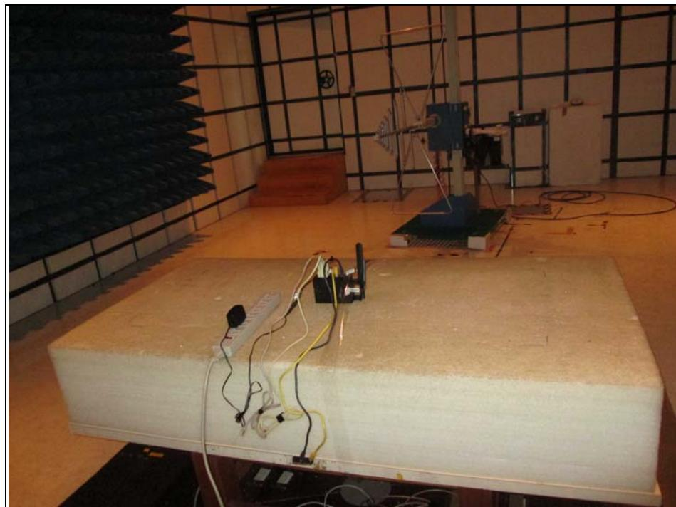
WWAN - Radiated Emission Test above 1GHz
