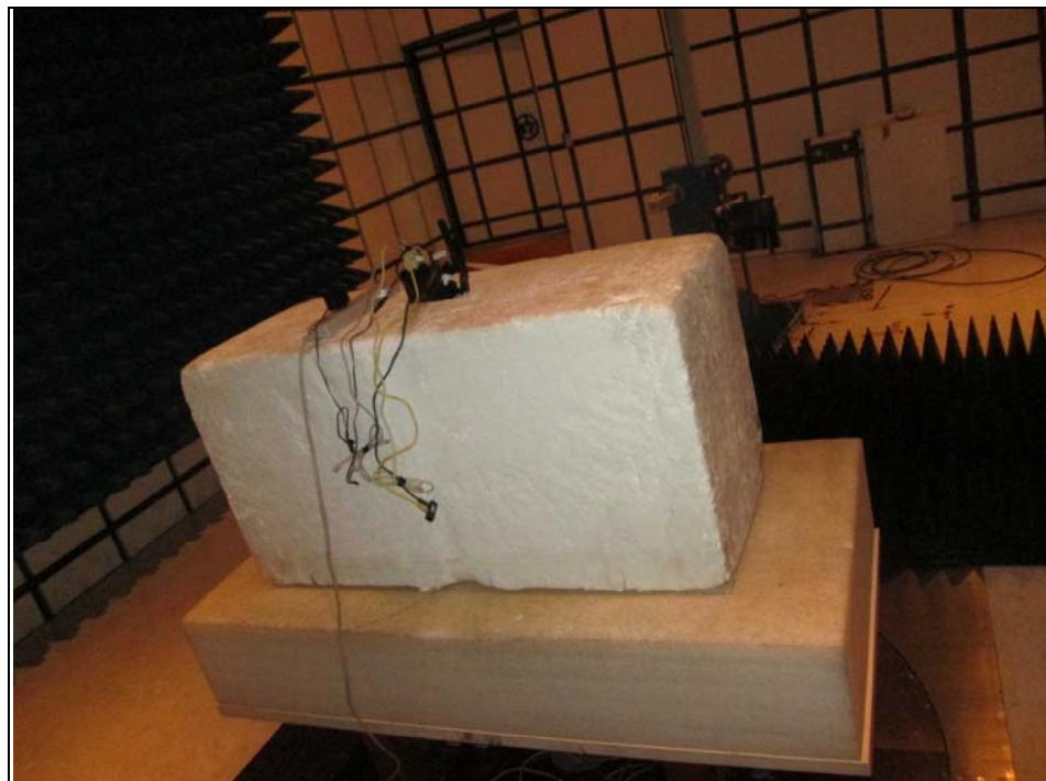
WLAN - Radiated Emission Test below 1GHz
