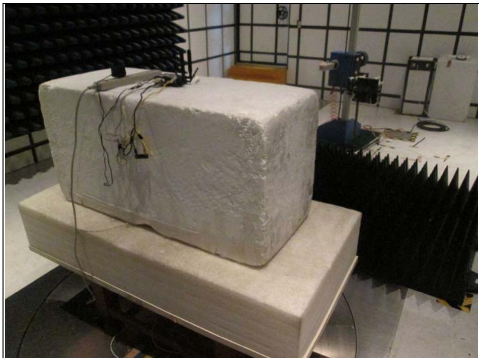
WWAN - Radiated Emission Test below 1GHz
