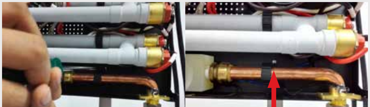
Figure 3. Tightening the Mounting Screws
