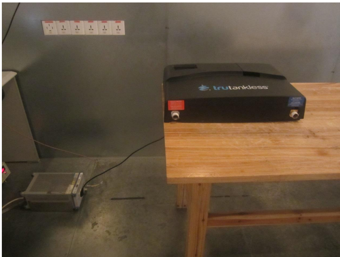
Conducted Emission at mains terminals
