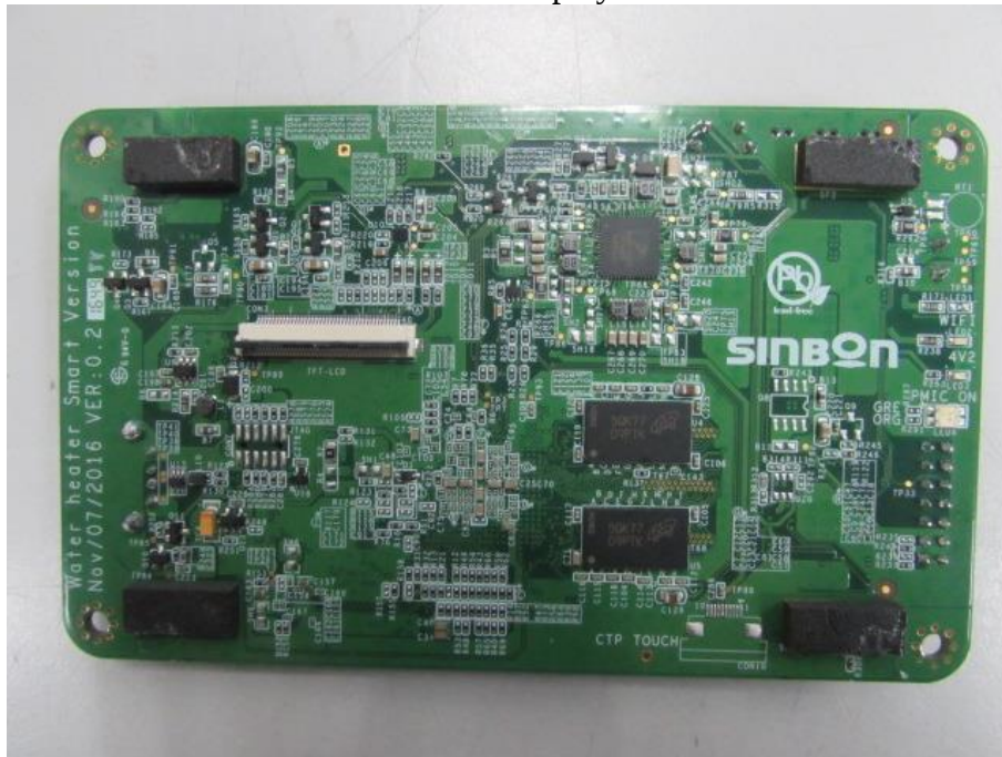
PCB view of display board
