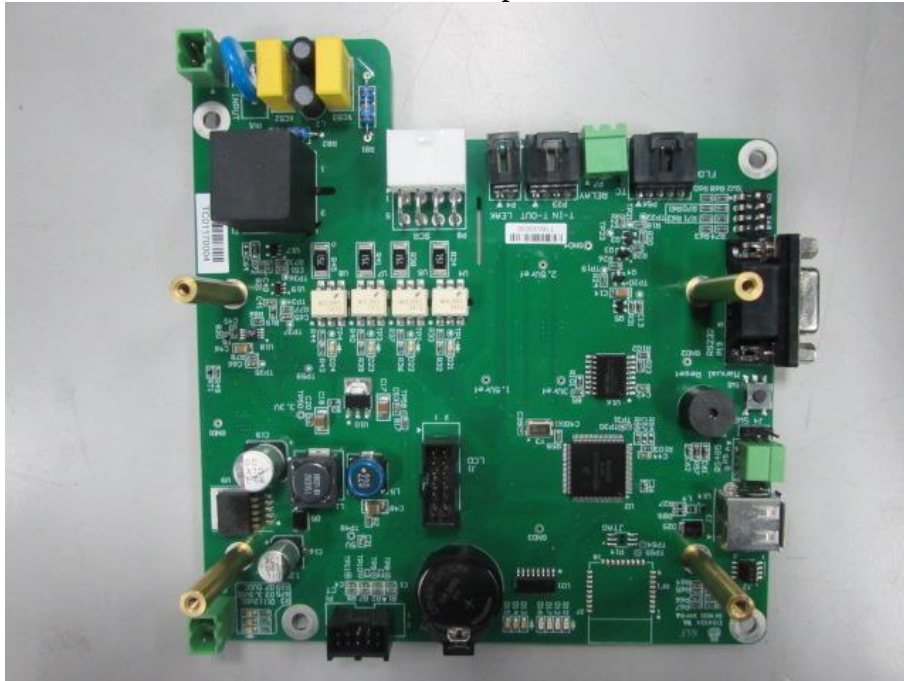
PCB view of main power board
