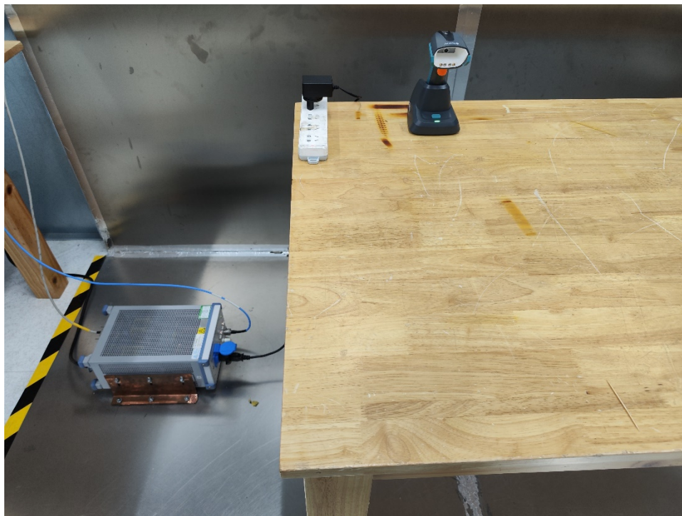
Photograph 3: Set-up for Conducted Emission on AC Mains
