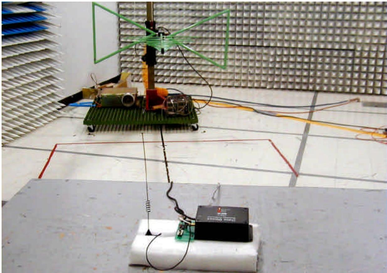
**Radiated Emissions Test Configuration**
