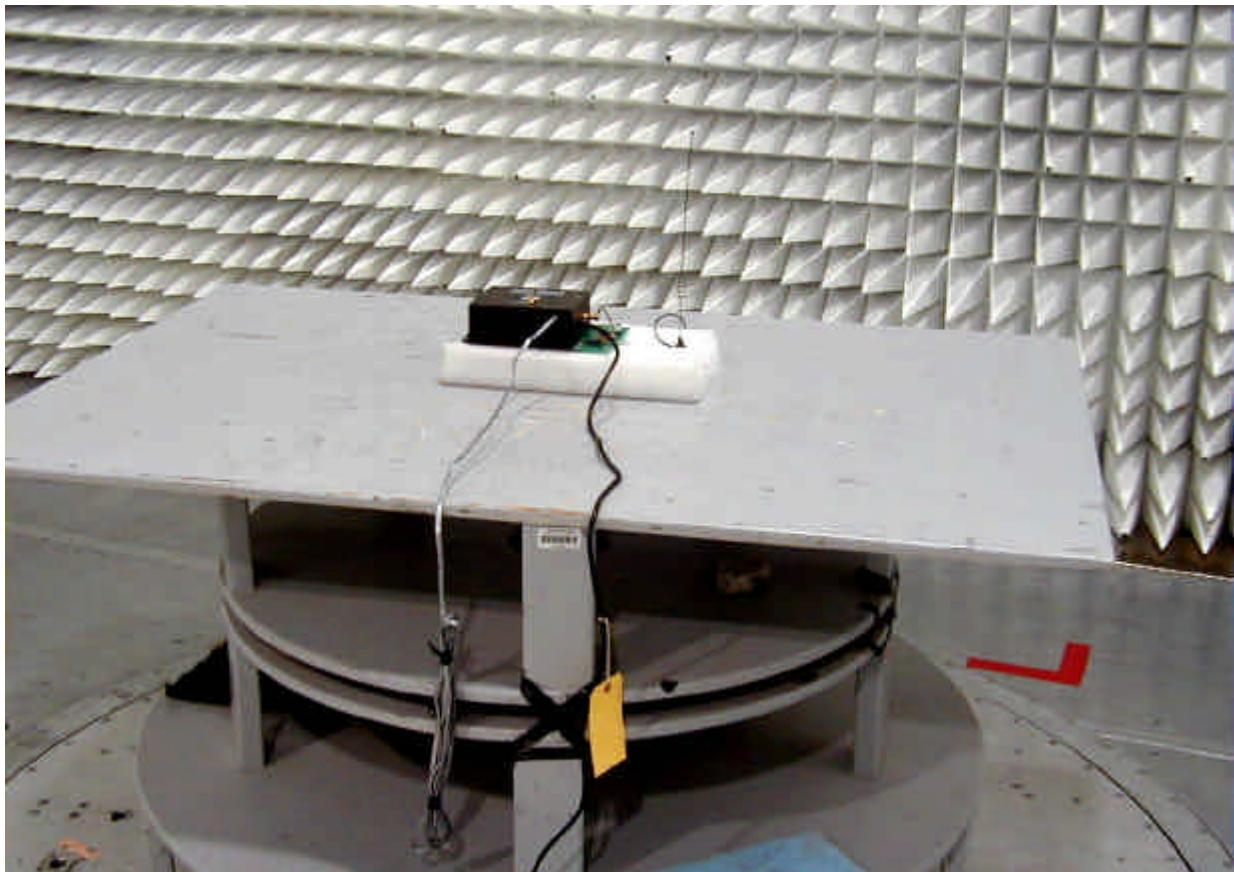
**Radiated Emissions Test Configuration**
