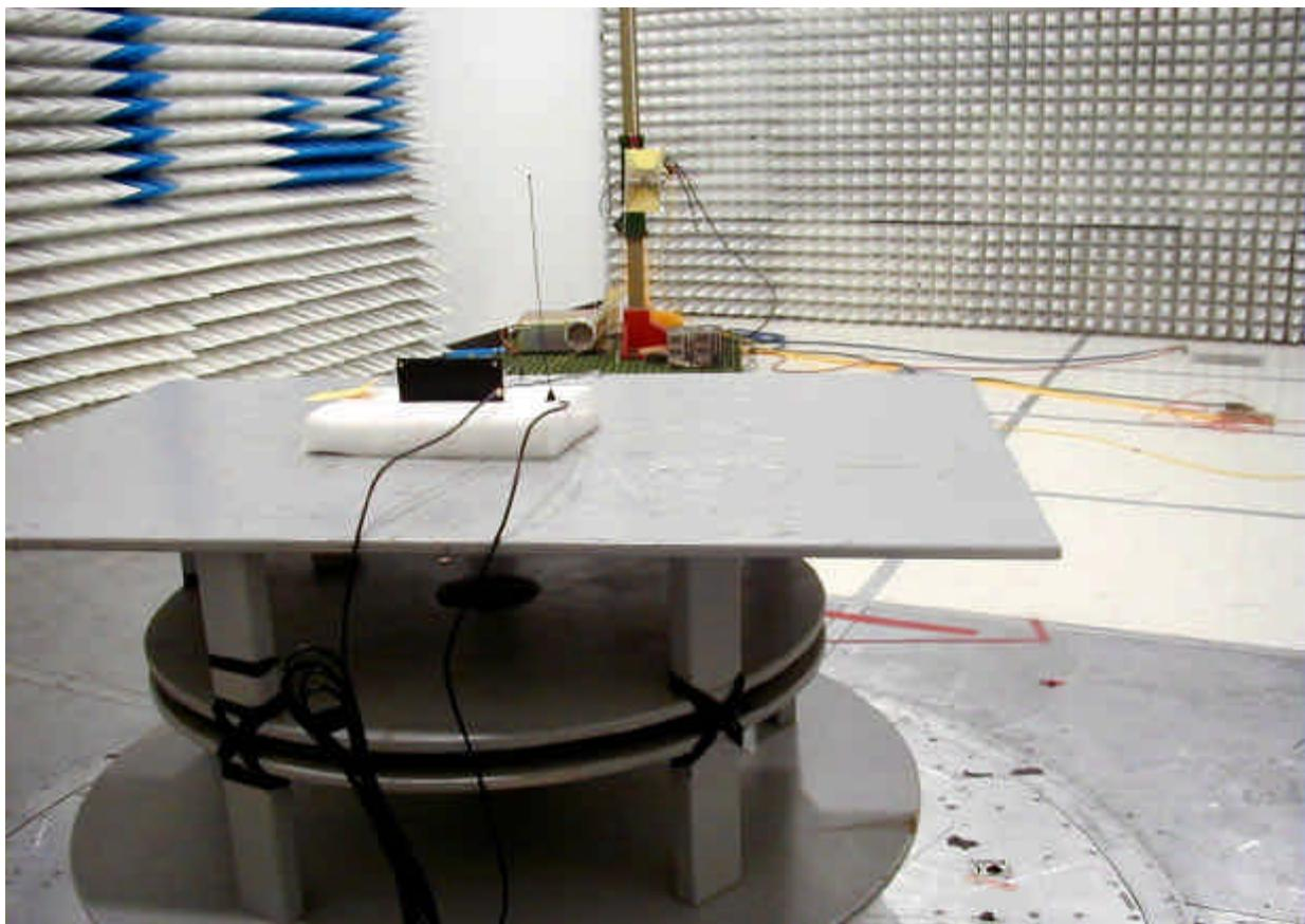
**Radiated Emissions Test Configuration**
