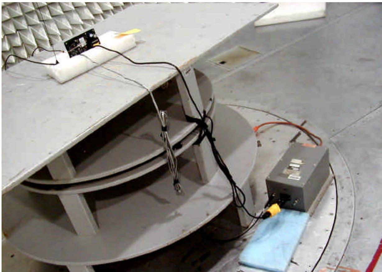
**Conducted Emissions Test Configuration**
