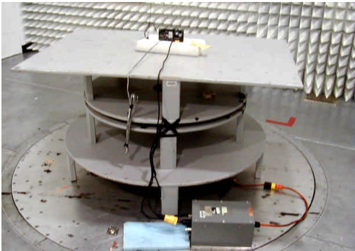
**Conducted Emissions Test Configuration**
