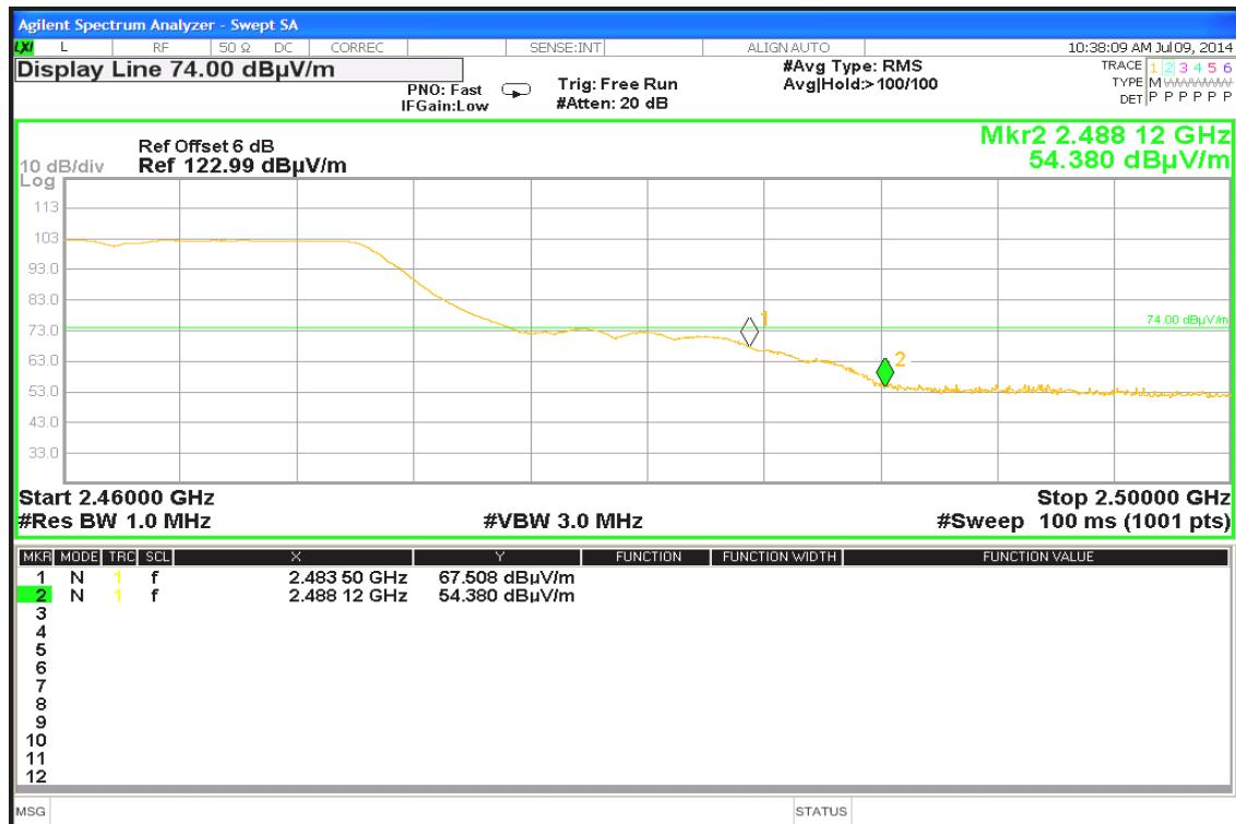
**Detector mode: Average****Polarity: Horizontal**
