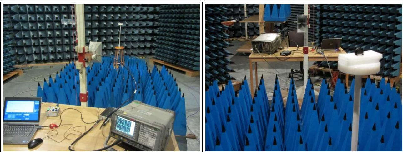
Remarks: Limit values expressed in dB $\mu$ V/m. The limit is 500 $\mu$ V/m at 3m;
