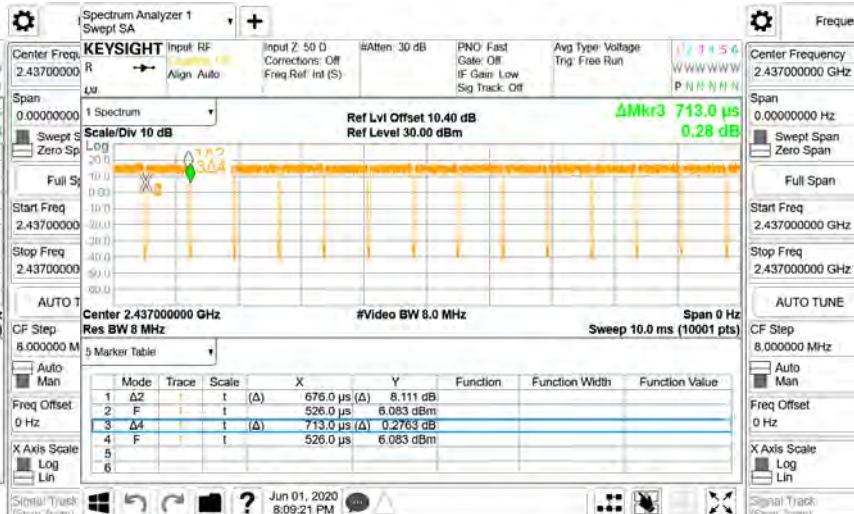
Duty Cycle 802.11n 40MHz 2437MHz
