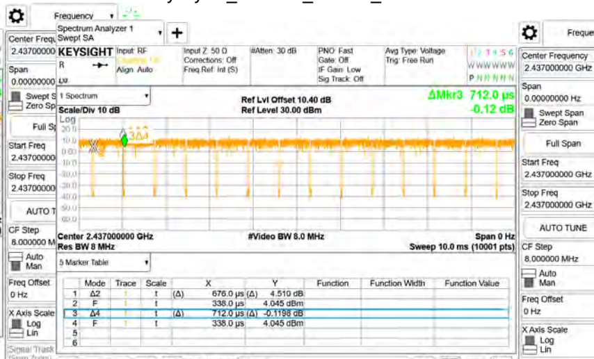
Duty Cycle 802.11n 40MHz 2437MHz
