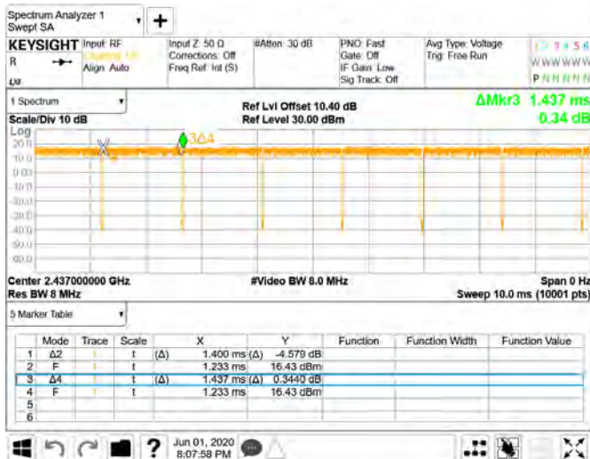
Duty Cycle_802.11g_20MHz_ 2437MHz
