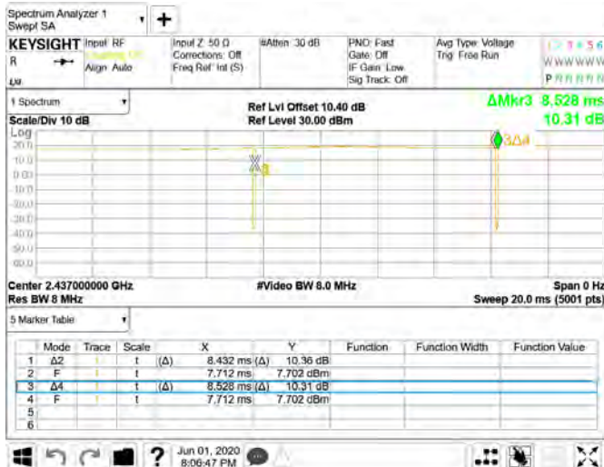
Duty Cycle_802.11g_20MHz_ 2437MHz
