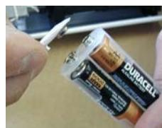
**Step 1:** Disconnect power (battery holder or power supply) from the Techniku motor, Intelligence Interface (I<sup>2</sup>) or standard receiver.
