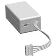
**Step 3:** Plug RF Module into Communication (COMM) port on Techniku motor or I<sup>2</sup>.
