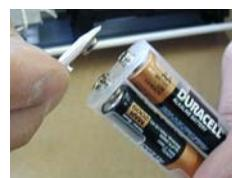
**Step 4:** Re-connect power (battery holder or power supply) to the Techniku motor or Intelligence Interface (I<sup>2</sup>). Power must be 6v, 12v or 24v.
