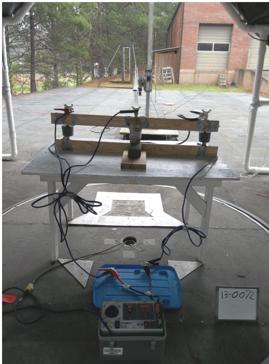
Photo 6 – Test Configuration of the EUT Digital Emissions, Rear View 200 MHz to 1 GHz Testing
