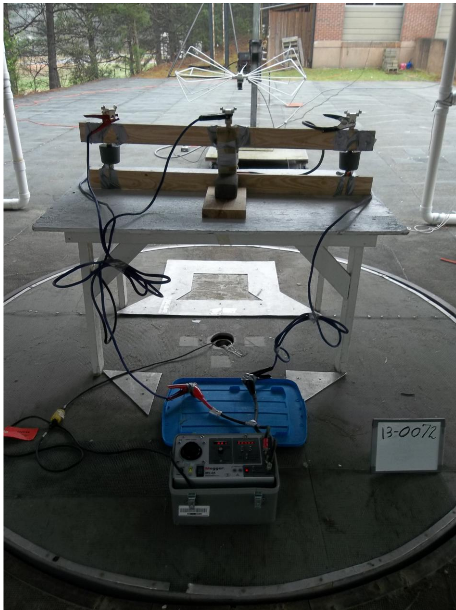
Photo 5 – Test Configuration of the EUT Digital Emissions, Rear View 30 MHz to 200 MHz Testing
