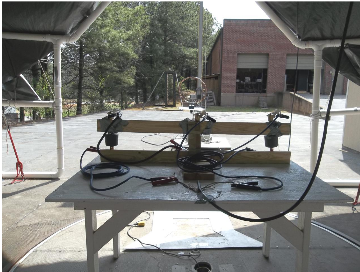
Photo 4 – Test Configuration of the EUT Digital Emissions, Rear View Below 30 MHz Testing
