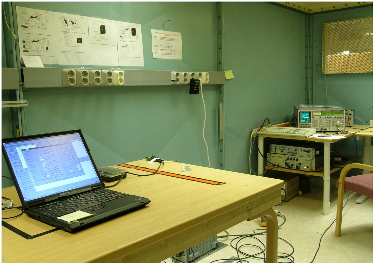
13213-SRB – Conducted emission test set-up
