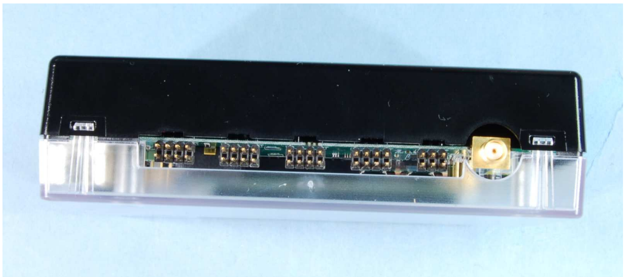
13213-NCB with plastic cabinet for radiated measurements
