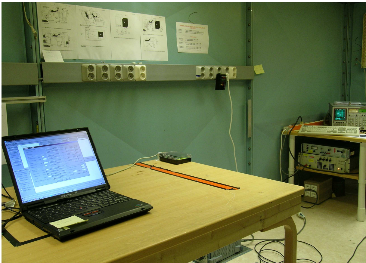
13213-NCB – Conducted emission – Test set-up
