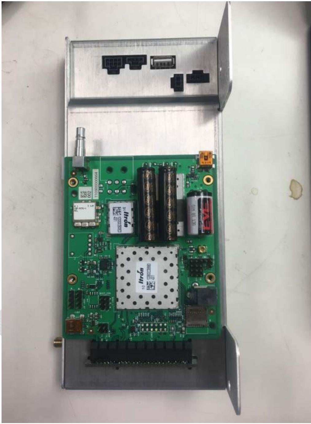
Install the shield that covers the NIC module with only RF QMA connect exposed.
