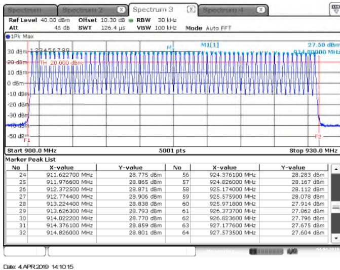
Figure 7.4.2.2-5: No. of Channels – DSSS – 12.5kbps
