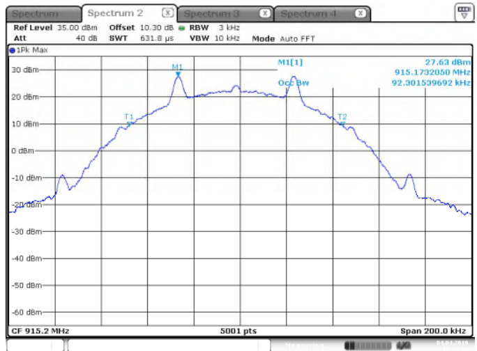
Figure 7.4.4.2-6: Sample Plot 99% OBW- FSK – 50kbps
