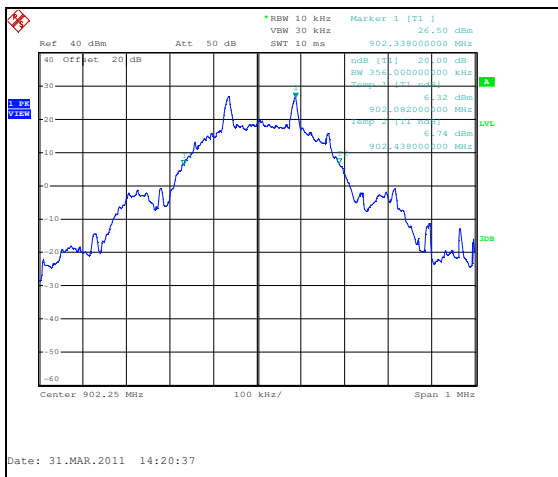
Figure 7.4.4.2-4: 20dB BW LCH – 152.3kbps
