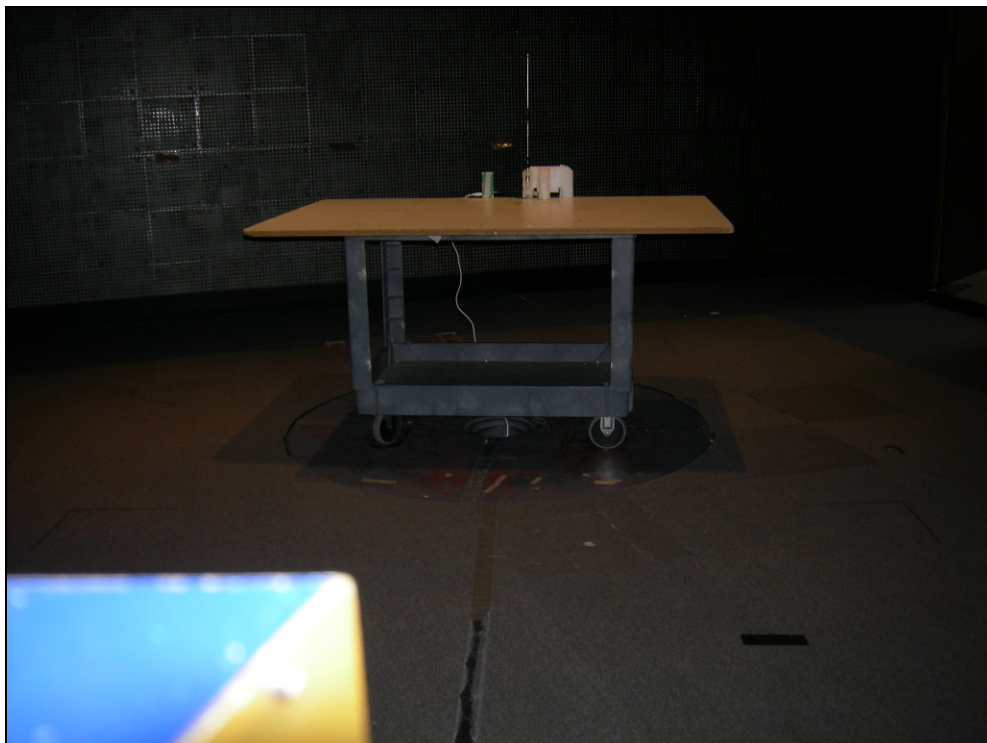
Figure 4: Radiated Emissions – Y-Pos
