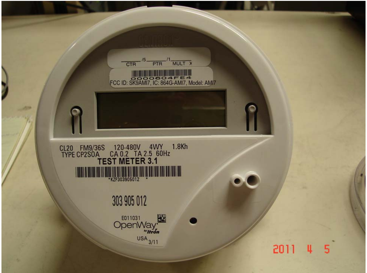
Figure 2: Itron AMI7 module installed in meter
