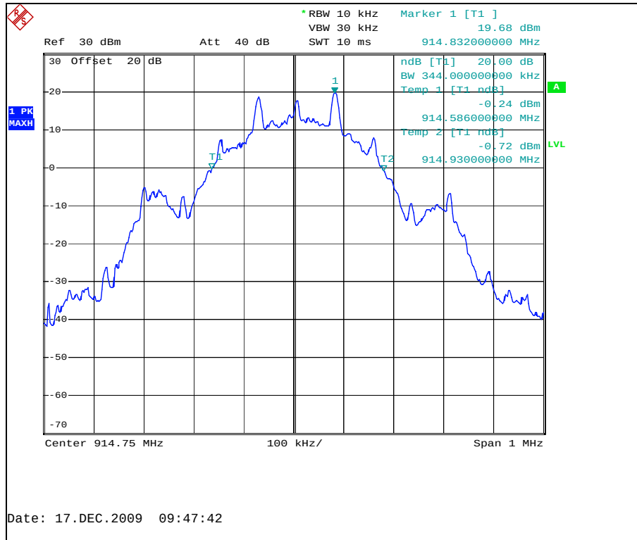
Figure 7.3.2-2: 20dB Bandwidth Plot – Mid Channel
