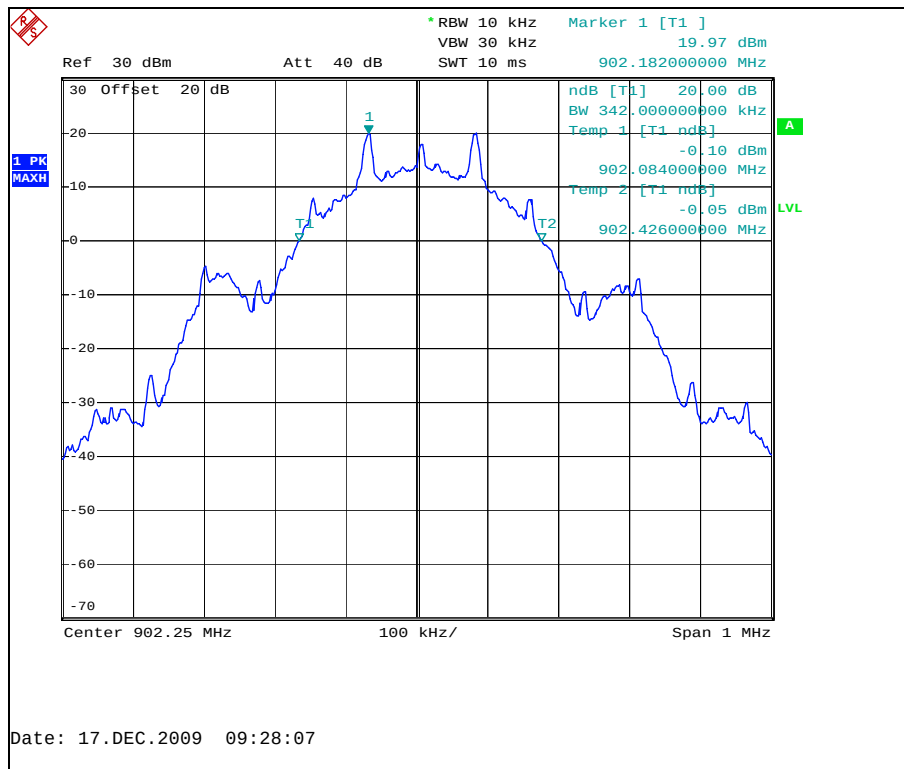
Figure 7.3.2-1: 20dB Bandwidth Plot – Low Channel
