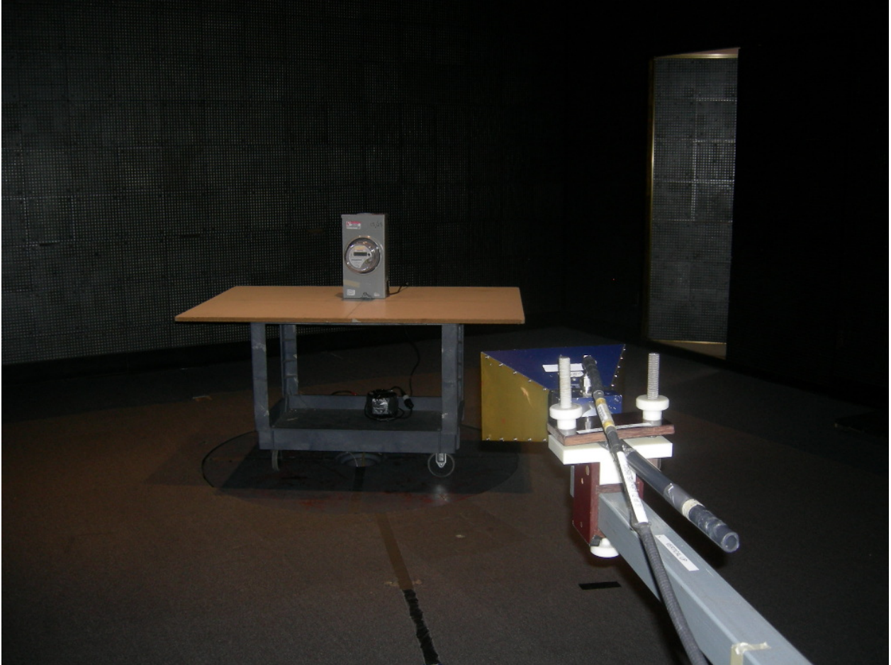
Figure 2: Radiated Emissions – Host 2S Meter Type
