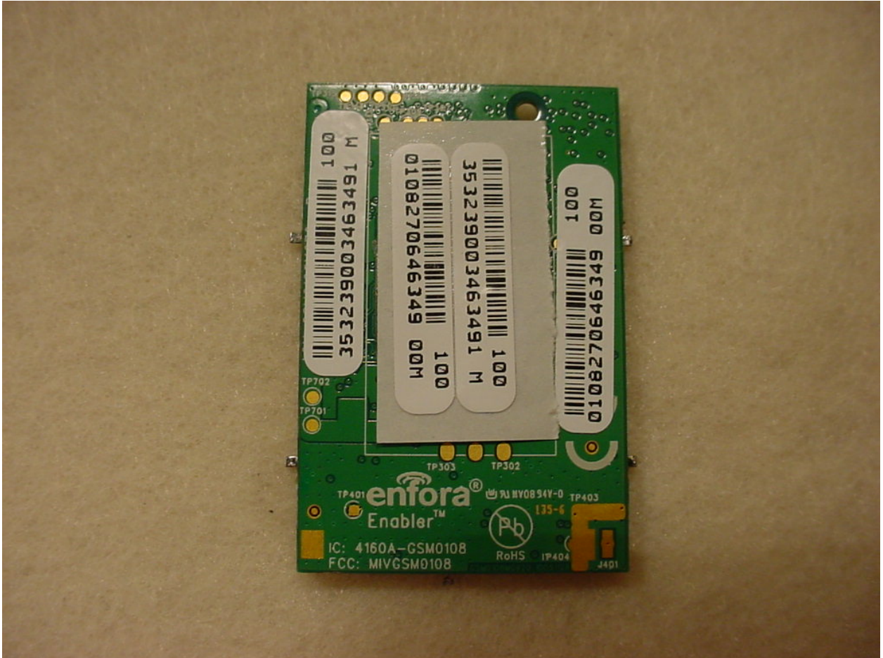
Figure 10: Internal –Enfora L.P. GPRS Modem Module Front
