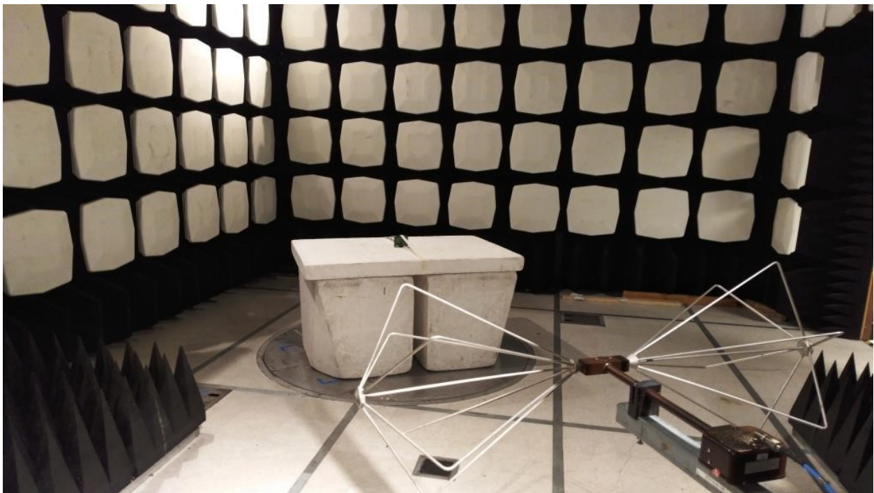
Figure 3: Equipment Under Test – Radiated Emissions – 30-1000MHz
