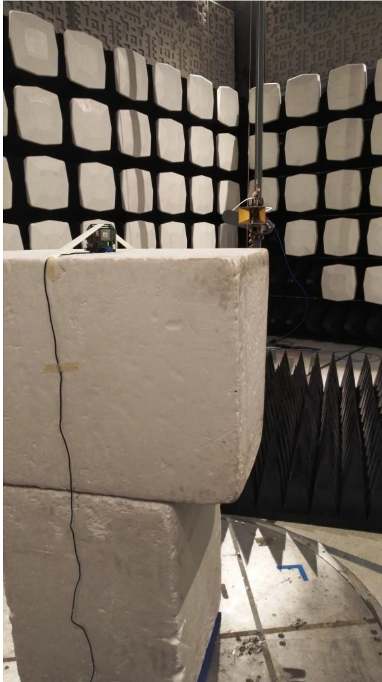
Figure 6: Equipment Under Test – Radiated Emissions – 1-18GHz
