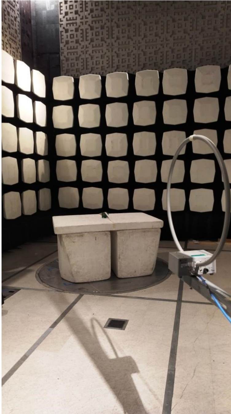
Figure 1: Test Setup – Radiated Emissions – Below 30MHz
