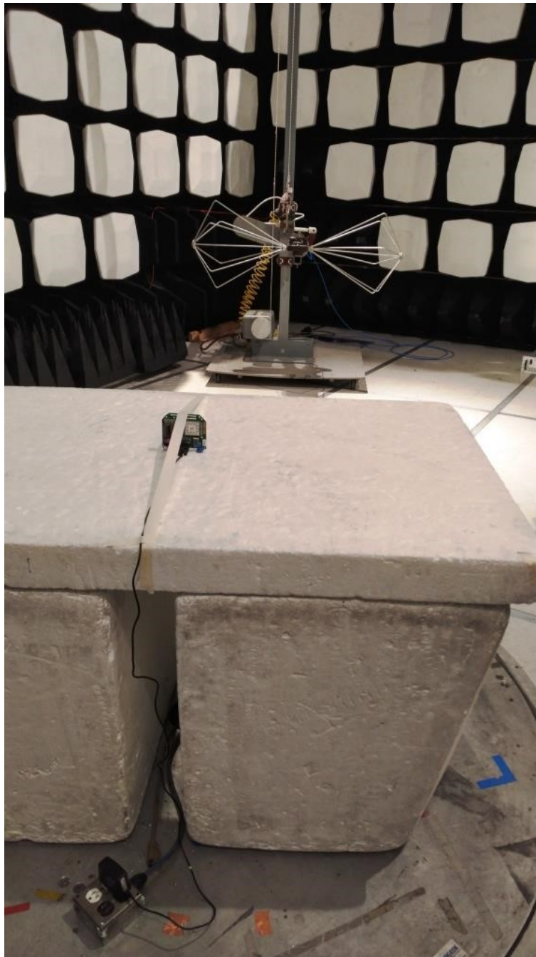
Figure 4: Equipment Under Test – Radiated Emissions – 30-1000MHz
