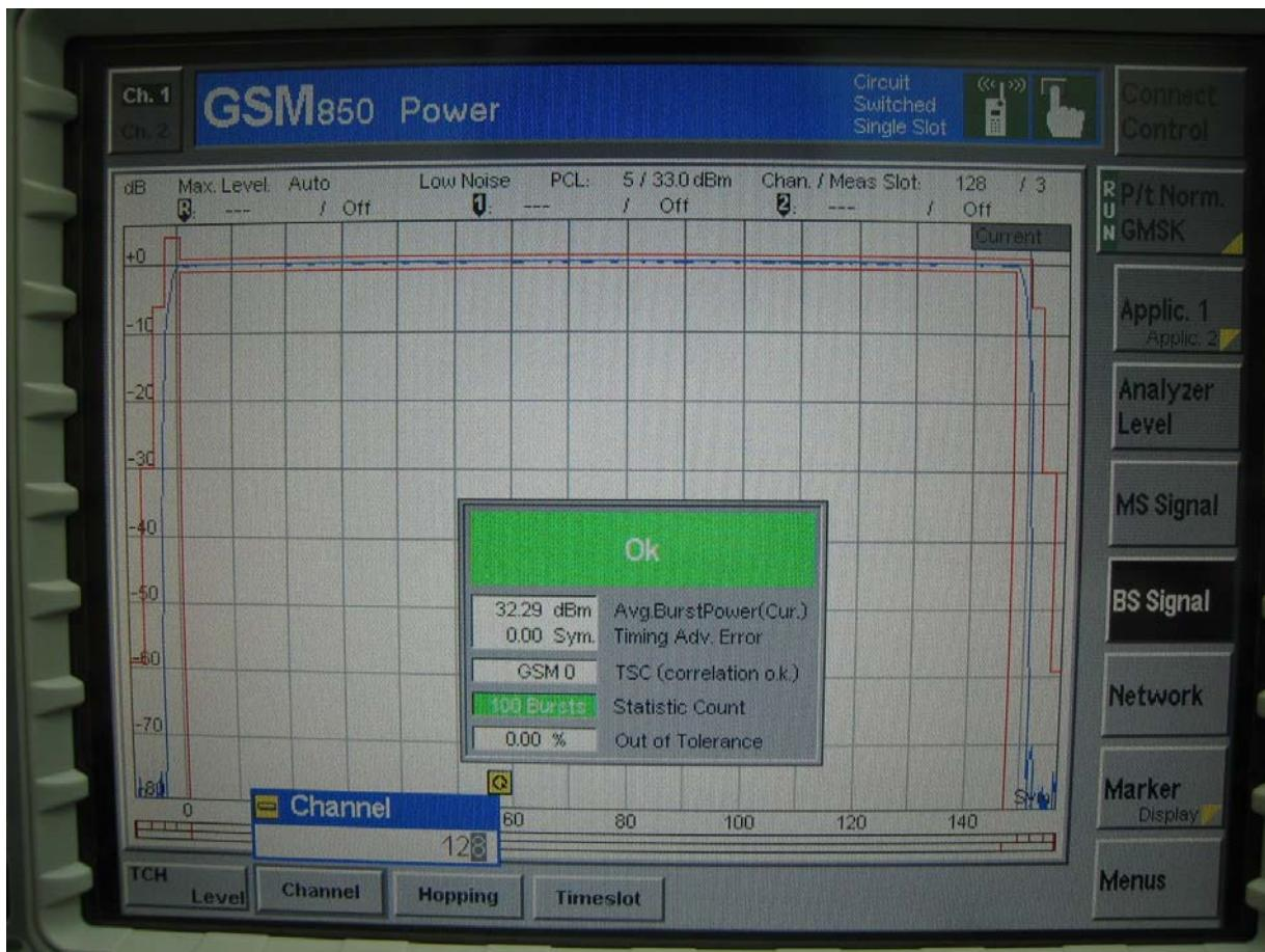
**■ Power output conducted (GSM850 190 CH)**
