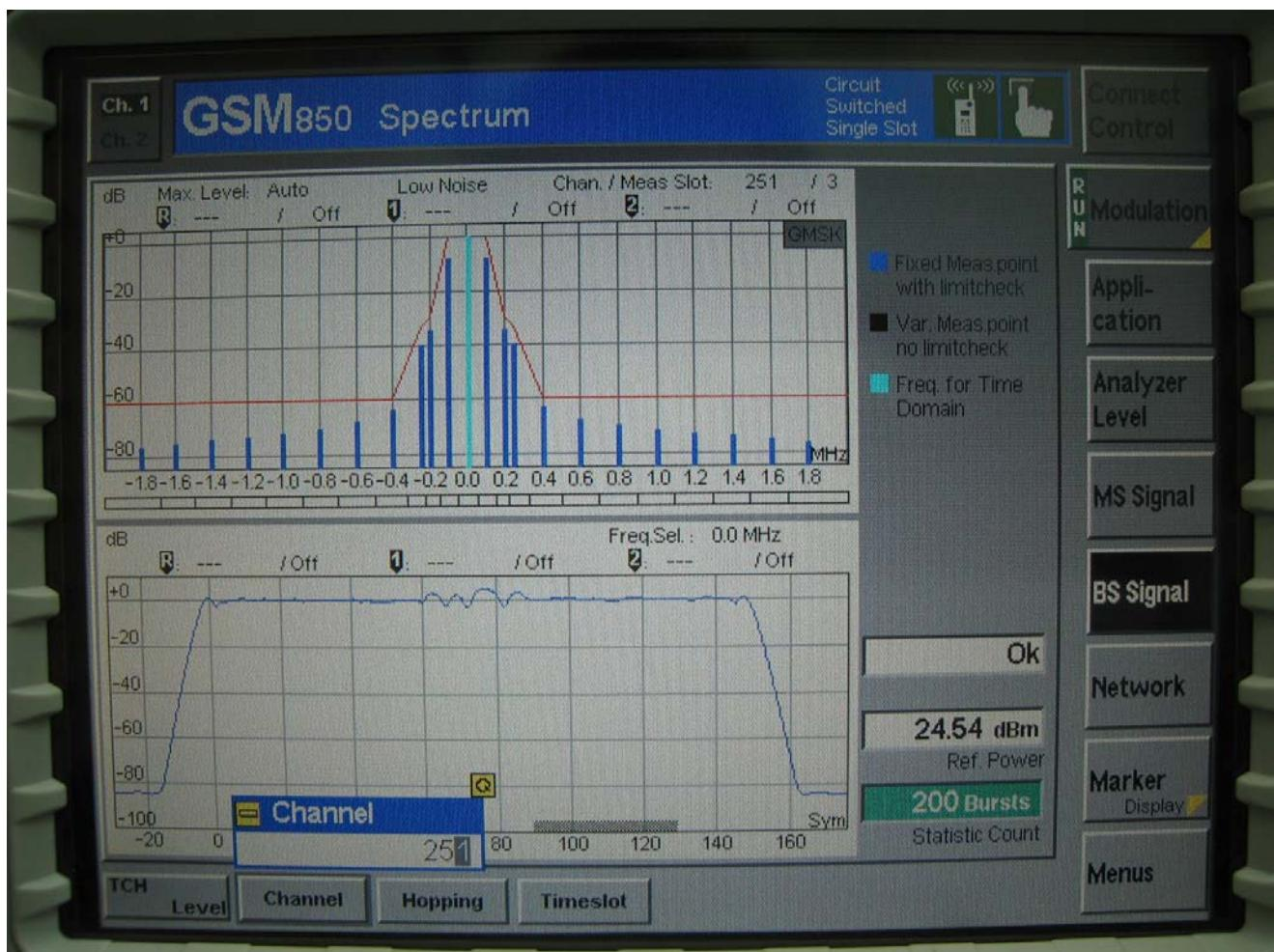
■ Modulation & Switching Graph (GSM1900 512 CH)
