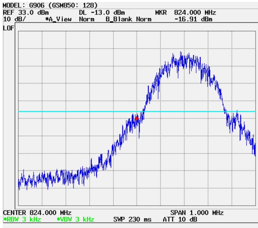
**■ GSM Block Edge GSM850 (251 CH.)**
