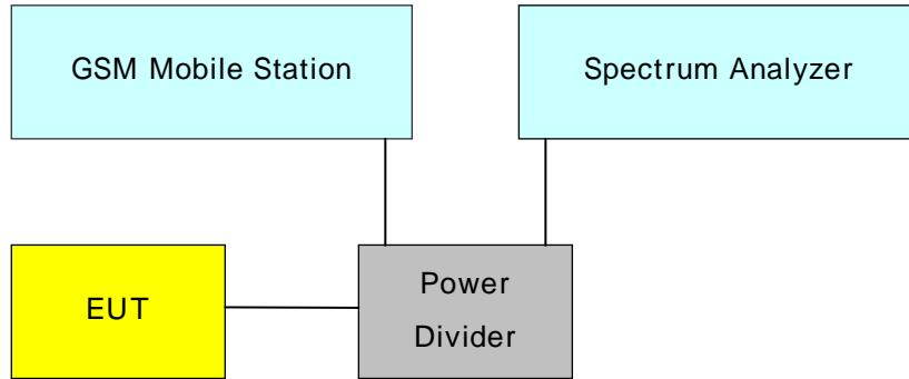
The level of the carrier and the various conducted spurious and harmonic frequencies is measured by means of a calibrated spectrum analyzer. The spectrum is scanned from the lowest frequency generated in the equipment up to 10 GHz. The transmitter is modulated with a 2500Hz tone at a level of 16dB greater than that required to provided 50% modulation.
