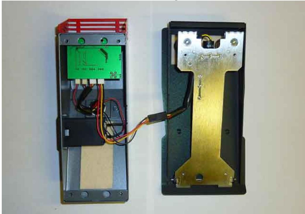
Internal view of electronics unit with PCB partially removed and turned over to view it's component side:
