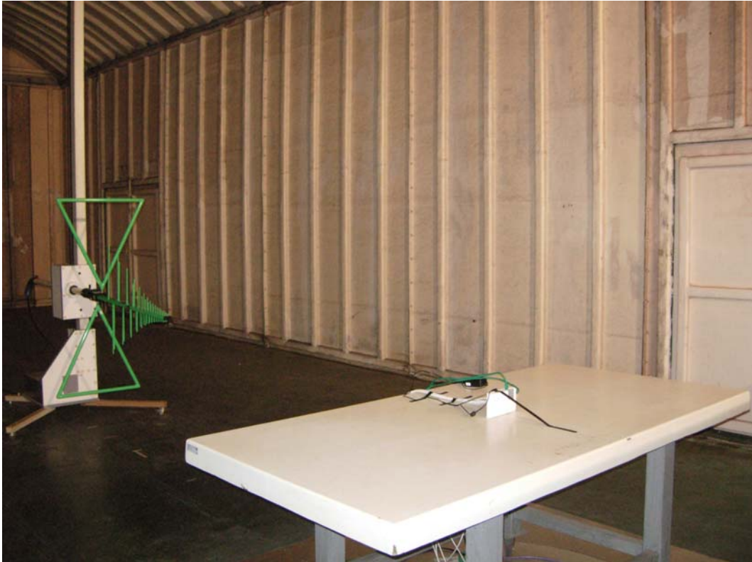
Front View of Radiated Test
