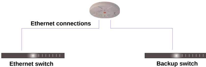
Figure 24. Switch Failover Protection
