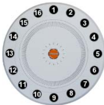
Figure 6. Layout of IAPs (XR-7630)
