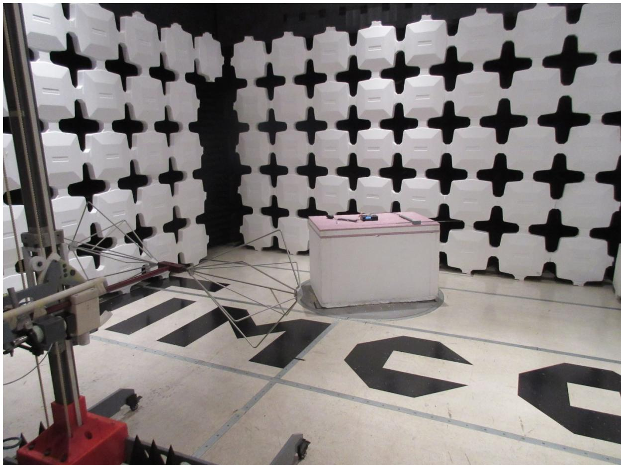
**Radiated Setup Below 200-1000 MHz**
