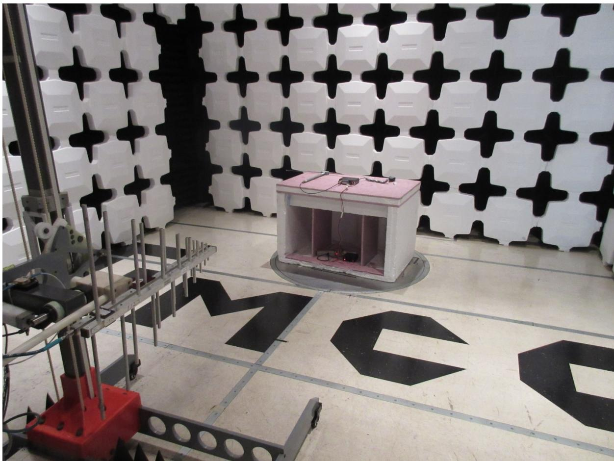
**Radiated Setup above 1GHz**
