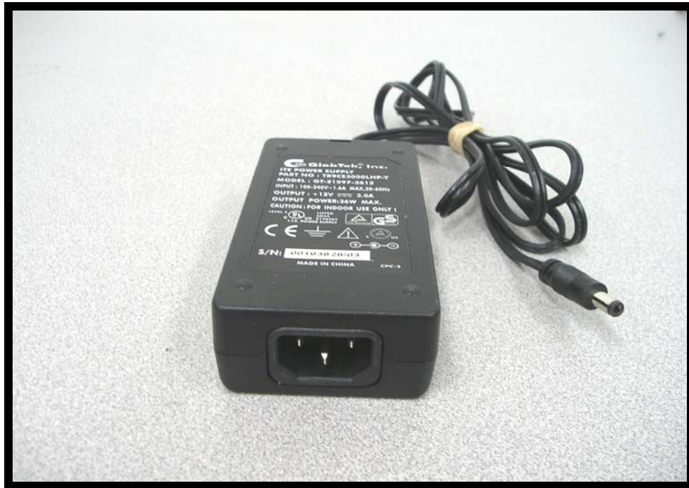
Figure 53: Power Supply for the EUT
