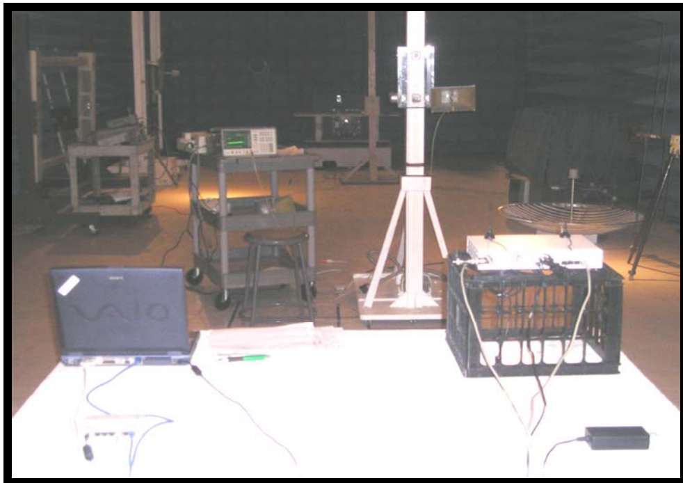
Figure 30: Rear View: Spurious Emissions test setup (Above 1 GHz)
