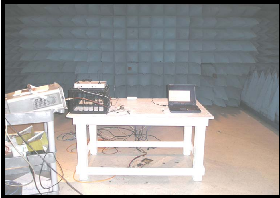
Figure 17: Peak Power Test Set-up Photo (Front View)
