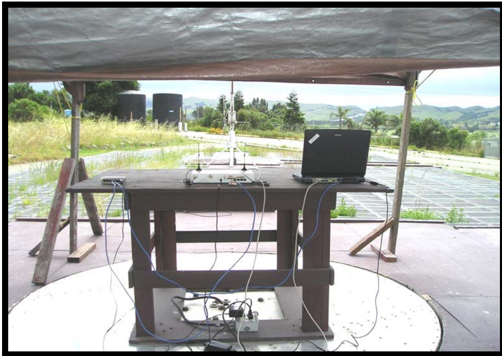
Figure 32: Rear View: Harmonic, Spurious test setup (Below 1 GHz)
