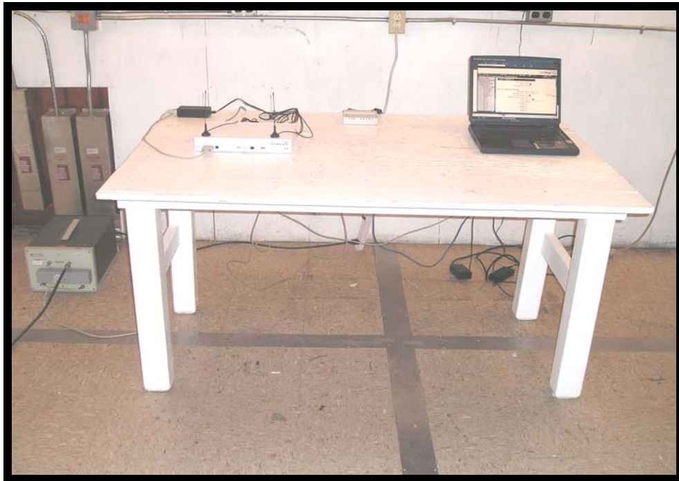
Figure 1: Power Line Conducted Maximized Emissions Test Setup (Front View)
