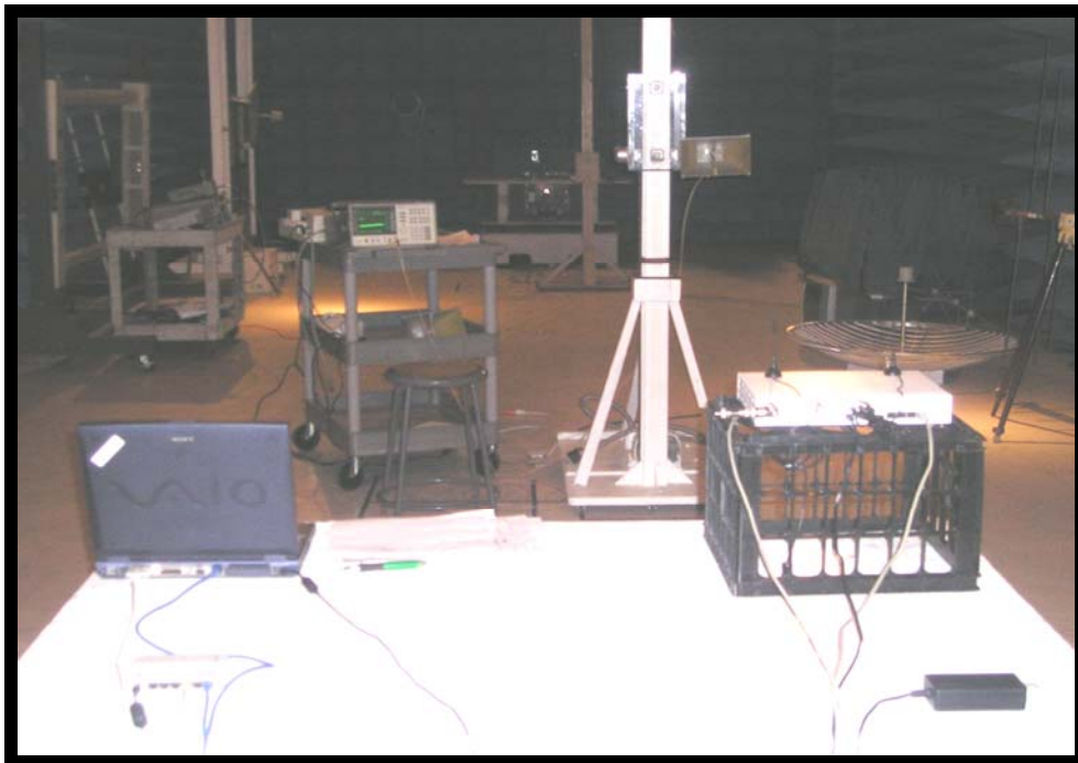
Figure 38: Rear View: Bandedge and restricted band measurement test setup.
