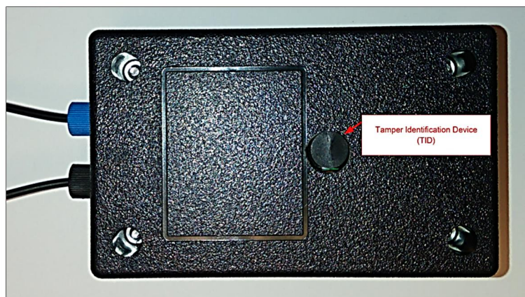
Figure 14 - Transmitter's Tamper Identification Device (TID)
