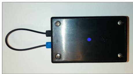
Figure 23 - Transmitter Status Lights – in Discovery mode
