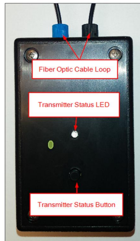
Figure 22 - Transmitter Status button and Status LED
