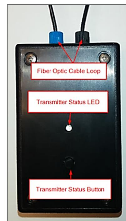
Figure 16 - Front with Status button & Status Led
