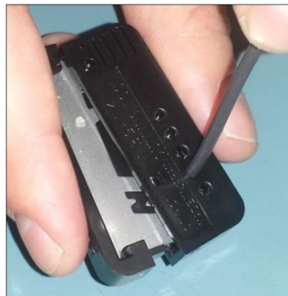
Figure 18 - Fiber optic cutter (Omron E39-F4)
