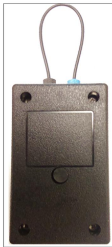
Figure 11 - Transmitter with fiber optic loop (back side)
