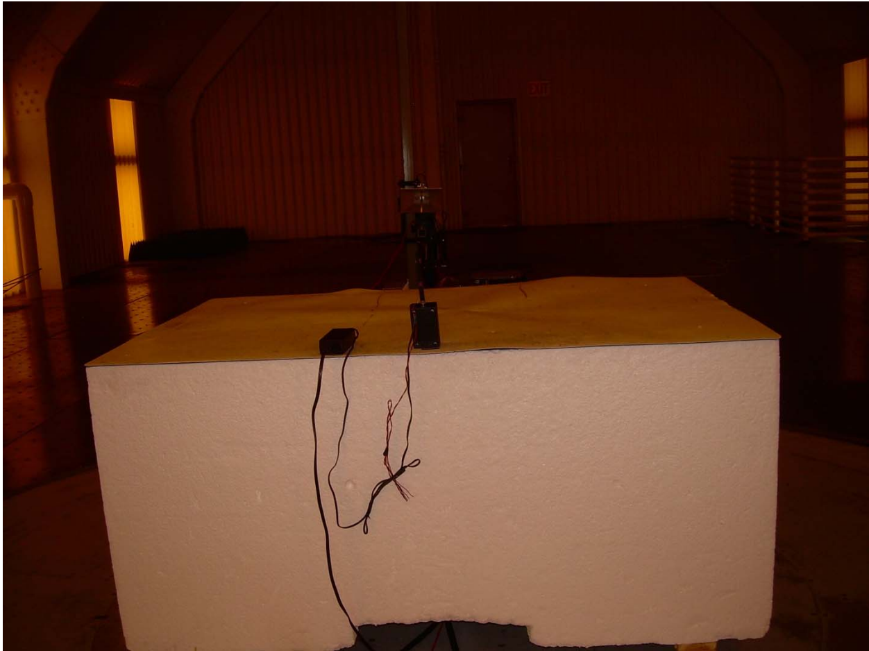
Photograph 2 – Front View Worst-Case Radiated Emissions Setup
