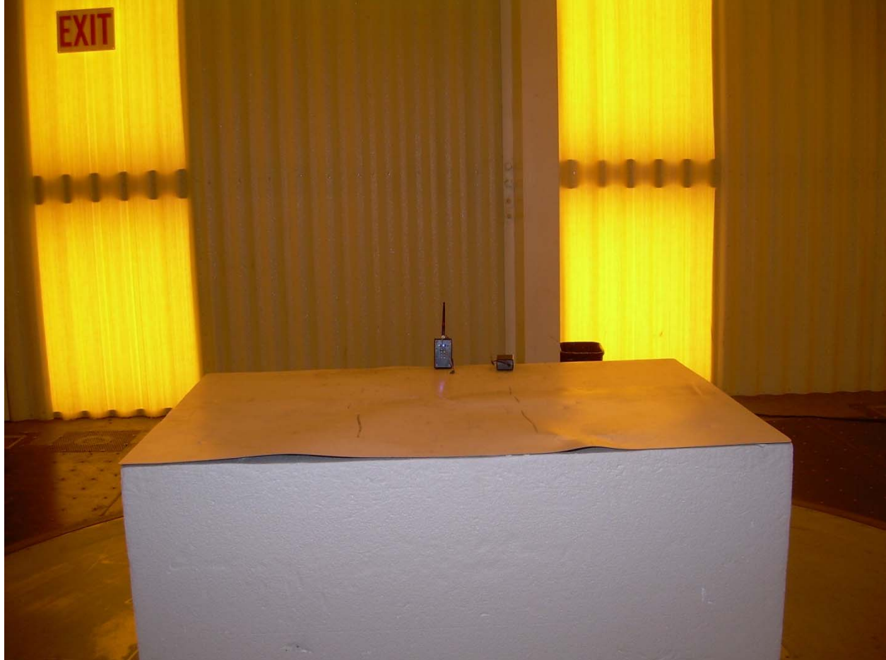
Photograph 1 – Front View Worst-Case Radiated Emissions Setup
